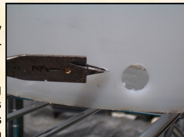
Hole in bucket with 1/2" wood drill bit. Tip courtesy of Carolyn Duncan — PLS.
